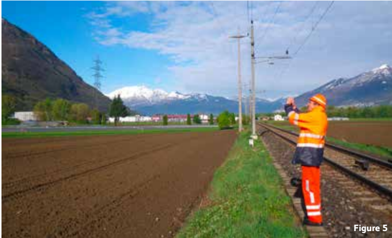
Recording the stray current distribution on the SBB network in Ticino
